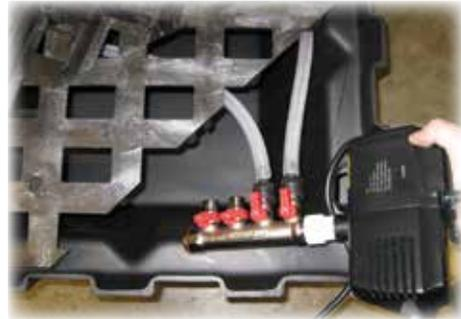
Plug the pump in and adjust valves as needed to desired effect before installing access door and decorative stone.
